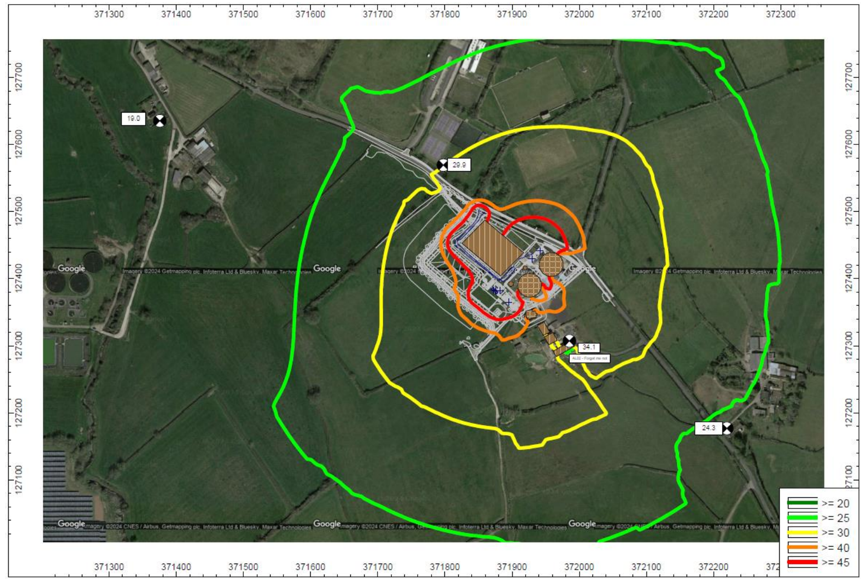
Figure B-1: Noise Contour Plot ( L_{Aeq} ) – Typical Daytime (1.5m)
