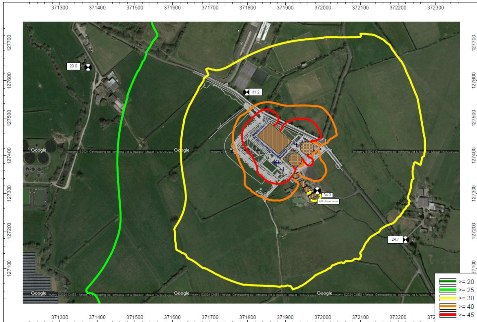
Figure B-3: Noise Contour Plot ( L_{Aeq} ) – Peak Daytime (1.5m)
