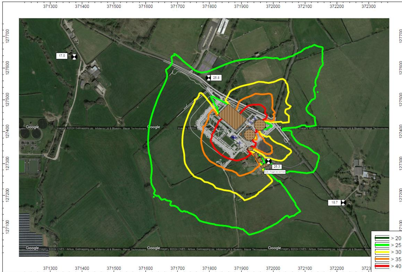
Figure B-2: Noise Contour Plot ( L_{Aeq} ) – Typical Night (4m)
