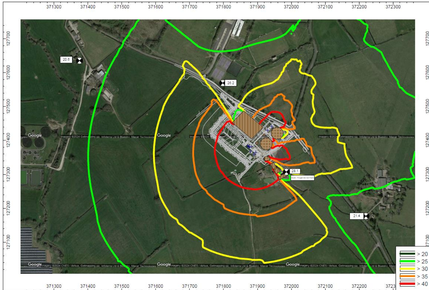
Figure B-4: Noise Contour Plot ( L_{Aeq} ) – Emergency Night (4m)
