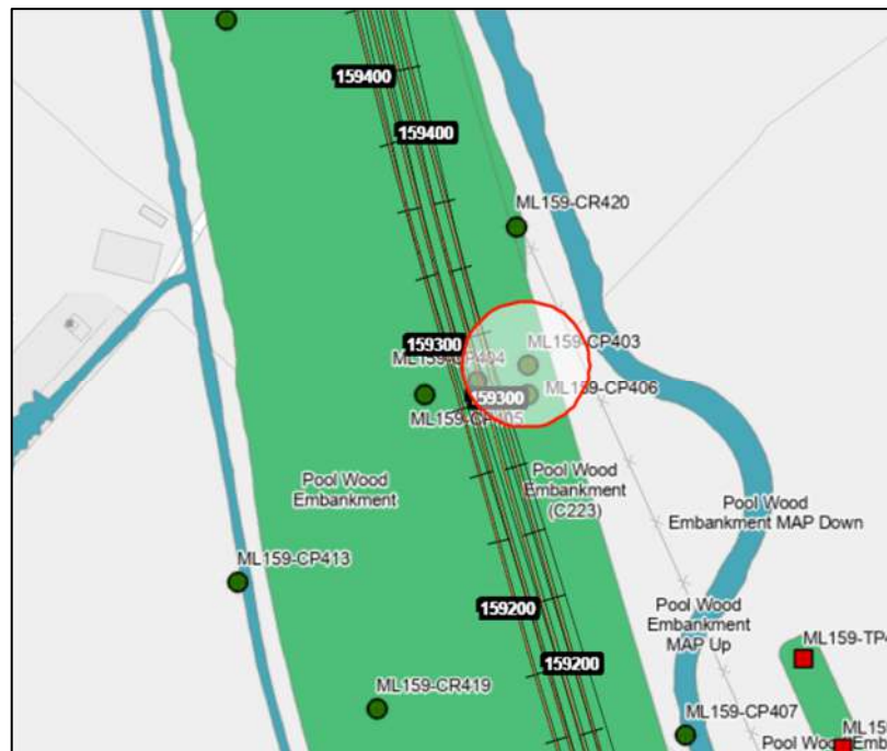
Figure 4: Location of soil lead and nickel exceedances above human health assessment criteria at Pool Wood Embankment
