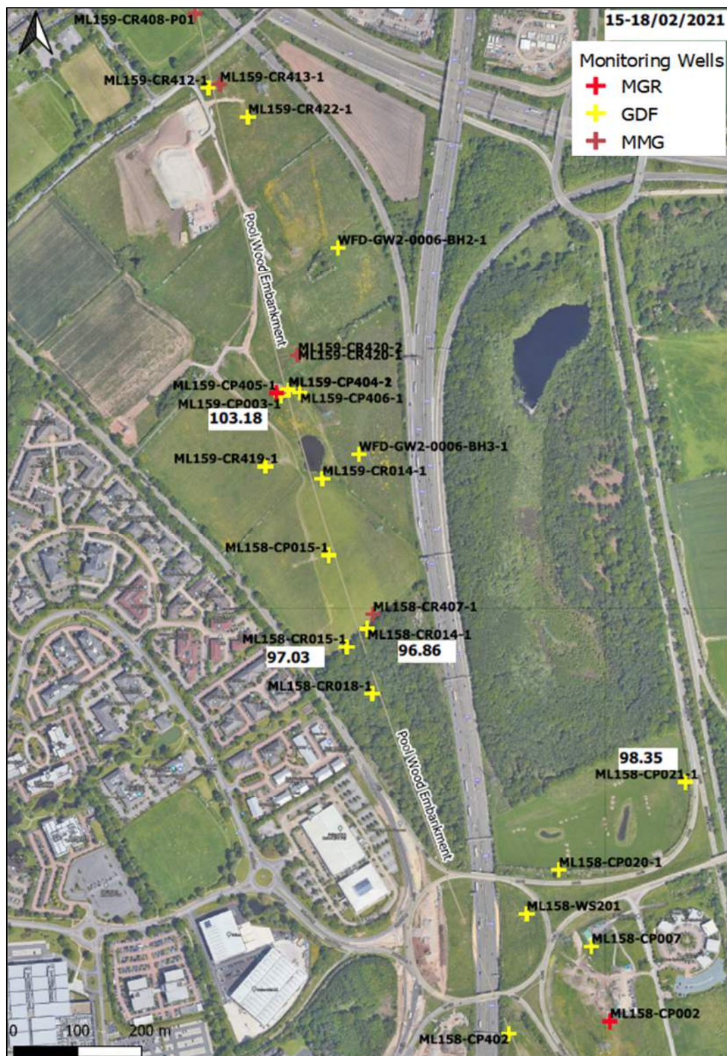
Figure 18 Groundwater elevations - February 2021 (mAOD)
