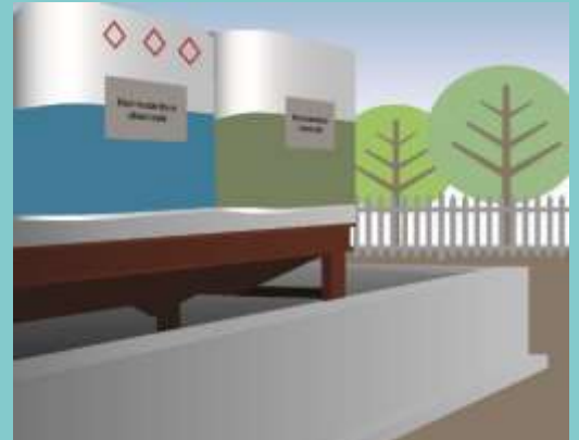
Illustration- chemicals stored in a bunded area to contain any spills
