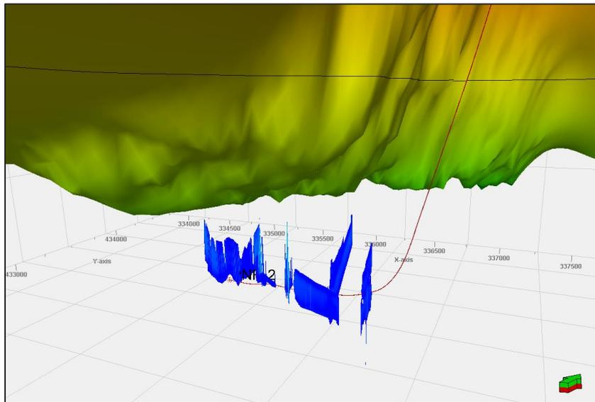
Cross sectional view looking due North across the PNR2 wellbore. The modelled fractures can be seen growing away from the well bore, this represents the complete fracture model not just the average fracture height. The upper limit of the permitted boundary is shown by the contoured horizon, green representing deep moving into yellow/red at shallower depths. A grid is provided for scale, each box has a side length of 500m
