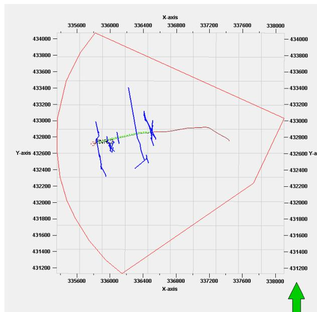
Map view of the permitted boundary, PNR2 wellbore shown in Dark red with Frac Stages shown in Green and the hydraulic fracture models shown in purple.
