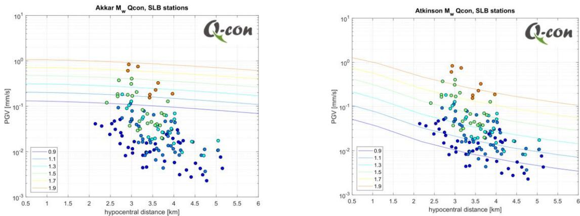
Measured peak ground velocity at SLB stations plotted against Hypocentral distance for the 19 events with  $M_L > 0$ . Magnitudes shown are  $M_w$  converted from  $M_L$ . Coloured dots denote measured values, binned to 0.1  $M_w$  intervals, taken as the maximum of the three-component recordings. Coloured lines denote predicted values according to Akkar et al (2014), left. Atkinson (2015), right. Local magnitude was converted to moment magnitude using the local  $M_L$ - $M_w$  conversion.
