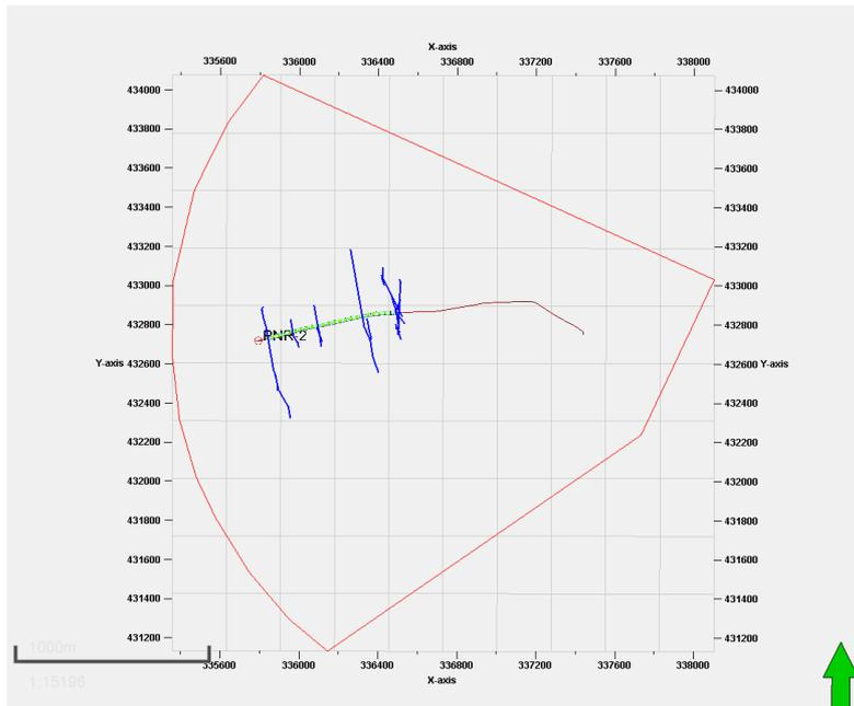
Map view of the permitted boundary, PNR2 wellbore shown in Dark red with Frac Stages shown in Green and the hydraulic fracture models shown in purple.
