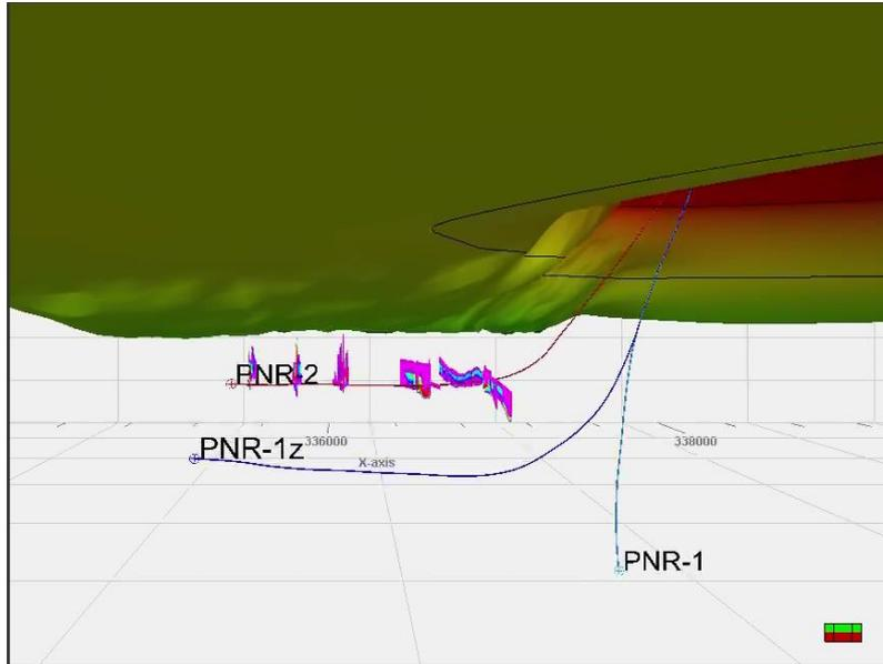
Cross sectional view looking due North across the PNR2 wellbore. The modelled fractures can be seen growing away from the well bore, this represents the complete fracture model not just the average fracture height. The upper limit of the permitted boundary is shown by the contoured horizon, green representing deep moving into red at shallower depths. A grid is provided for scale, each box has a side length of 800m.
