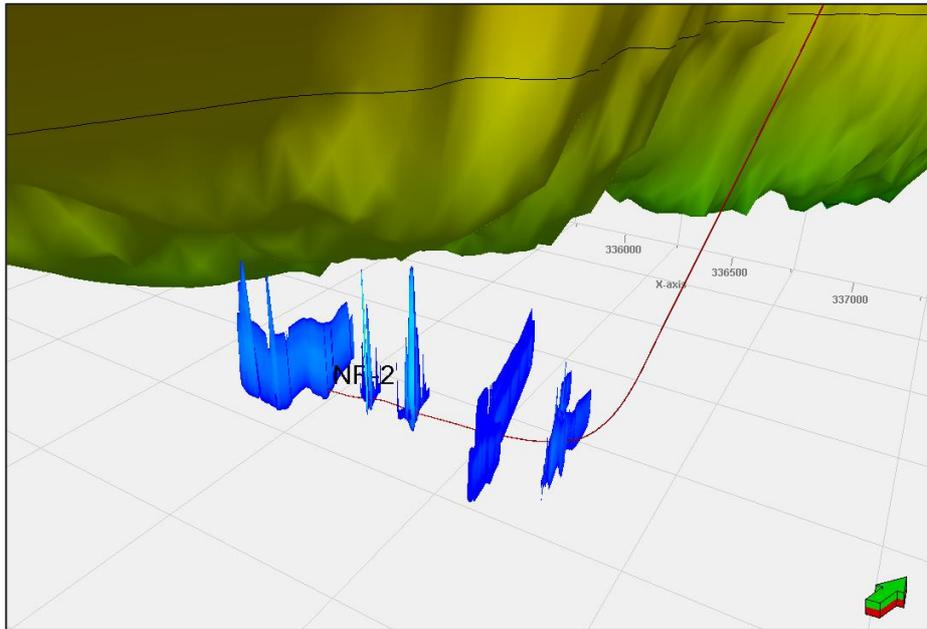
\* Clarification note: cross sectional orientation gives a view of fractures into green zone. This is incorrect due to the orientation of the view and not a permit breach. Confirmation is provided in section m, Kinetix table of frac height growth (gel injection).
