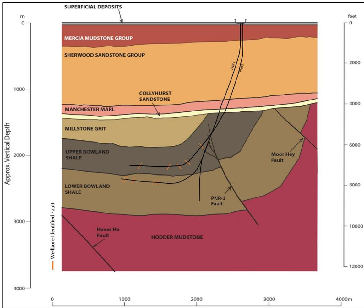
MS\_PNR1z\_ii feature projected onto cross section following PNR2 well profile
