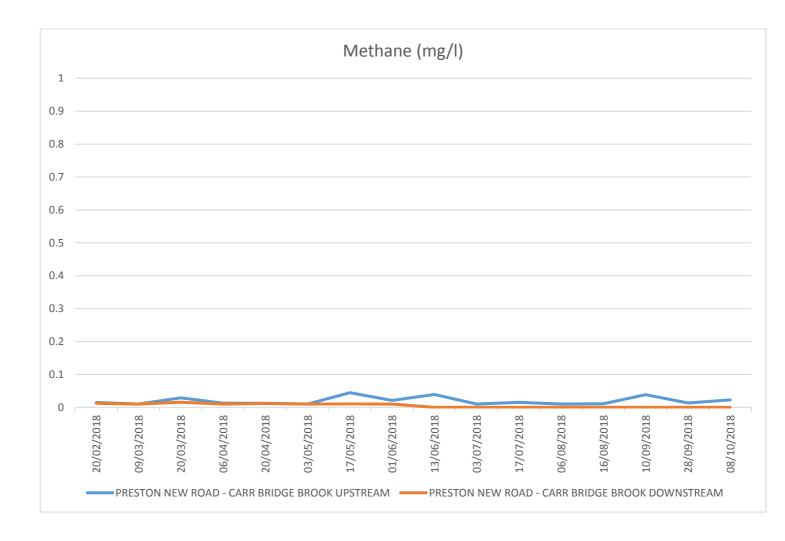
All results prior to 20 February 2018 were less than 0.5 mg/l which was the limit of detection at the time.
