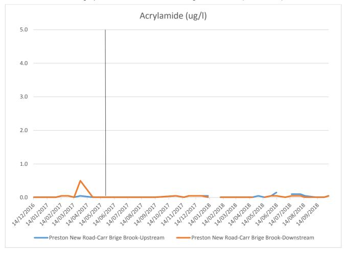
Limit of detection was 0.5 ug/l or below depending on quality of the sample received. Spike shown on 29 March 2017 was a poor quality sample and therefore the limit of detection was compromised. No Acrylamide was being used on site at the time. As a reference, the drinking water standard is 0.1 ug/l.
