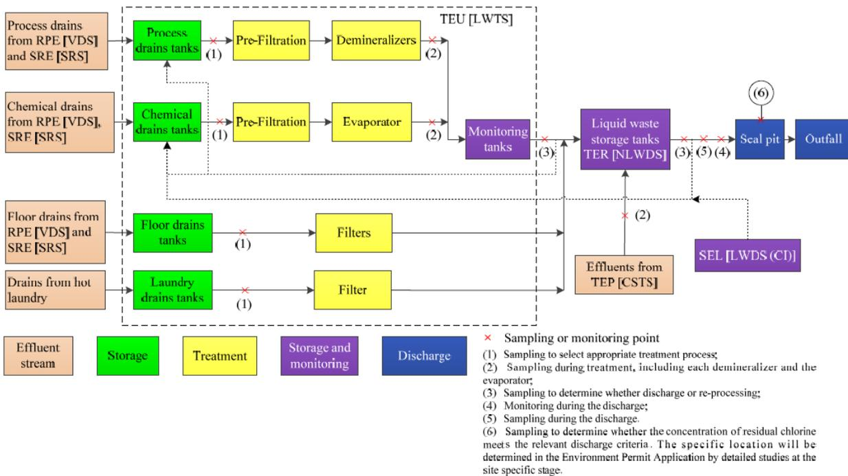
**Figure 1: GNSL flow diagram for liquid radioactive effluent streams (GNSL, 2020b)**
