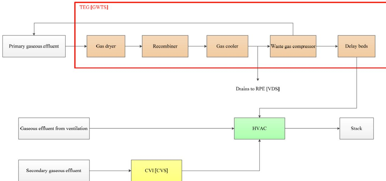
**Figure 2: Radioactive gaseous effluent streams (GNSL, 2020b)**
