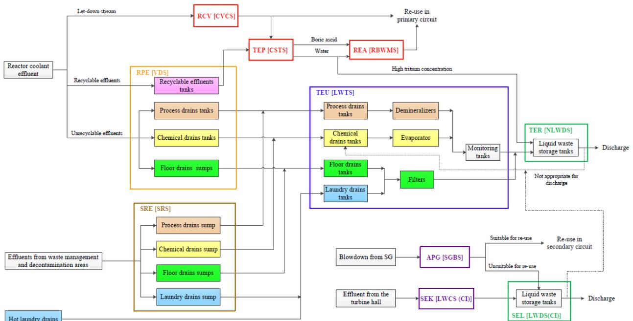
**Figure 3: Liquid effluent streams and LRWMS (GNSL, 2020b)**
