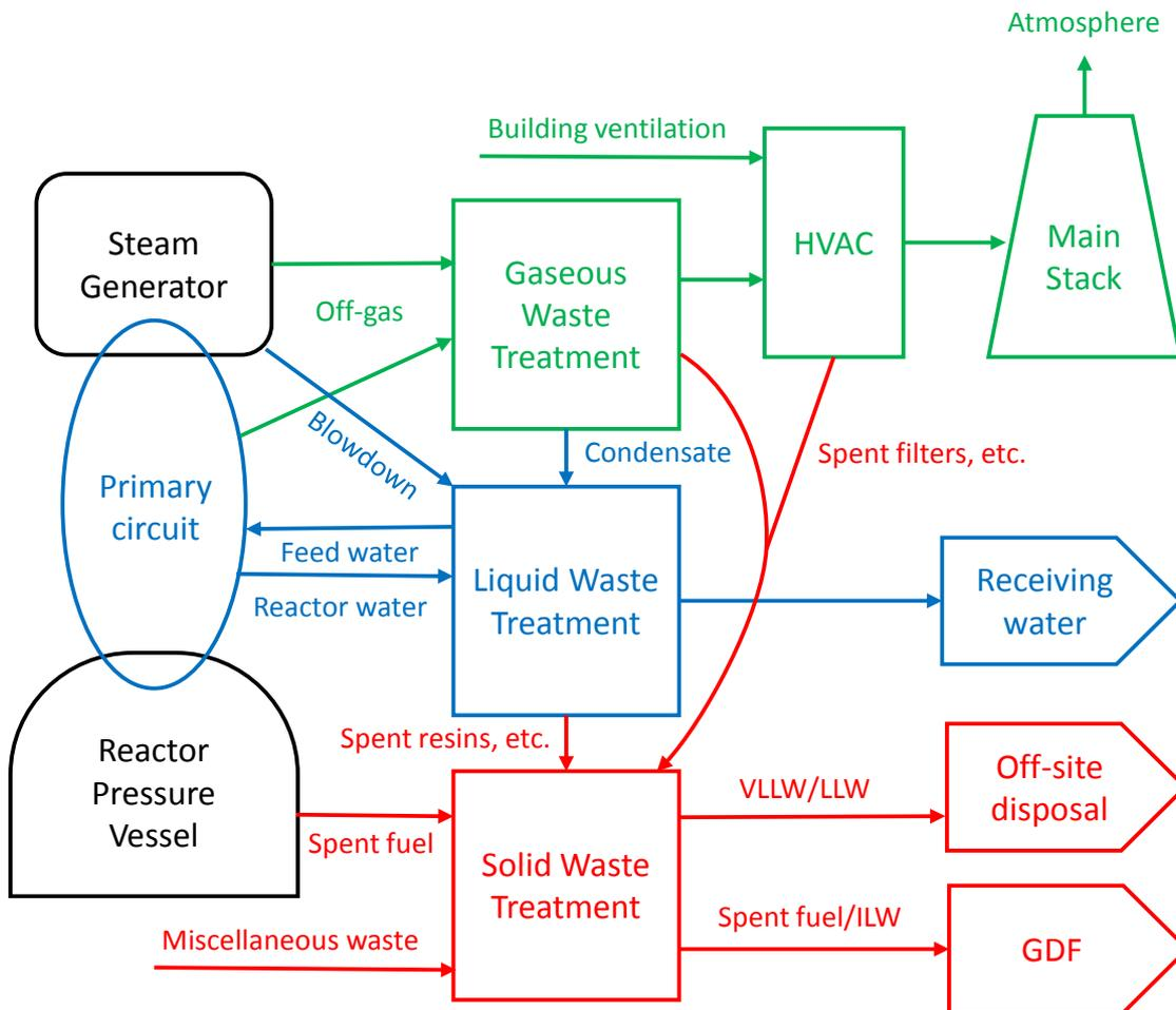
**Figure 1: The gaseous, liquid and solid wastes routes.**
