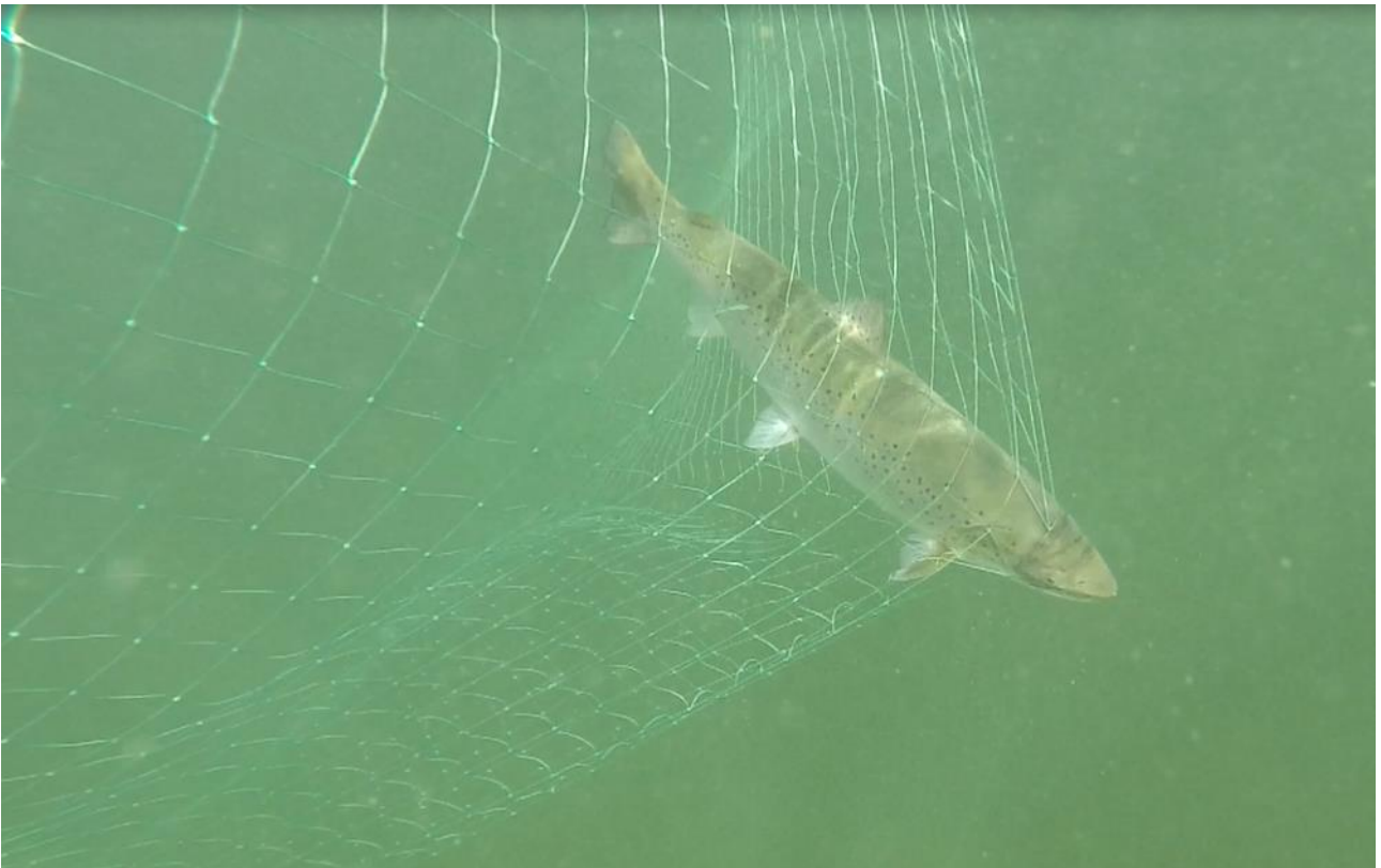
4. Sea trout entangled in the head piece of the modified T net
