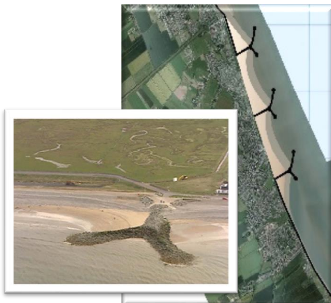
Visualisation of how a fishtail groyne may look on the Lincolnshire beaches
