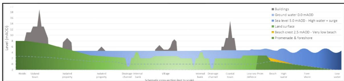
Figure 3: Schematic cross-section of the Lincolnshire flood plain without a flood defence
