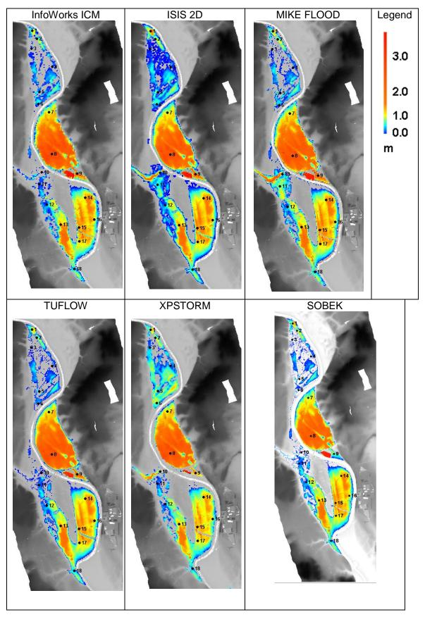
Figure 4.39 Final depths predicted in Test 7
