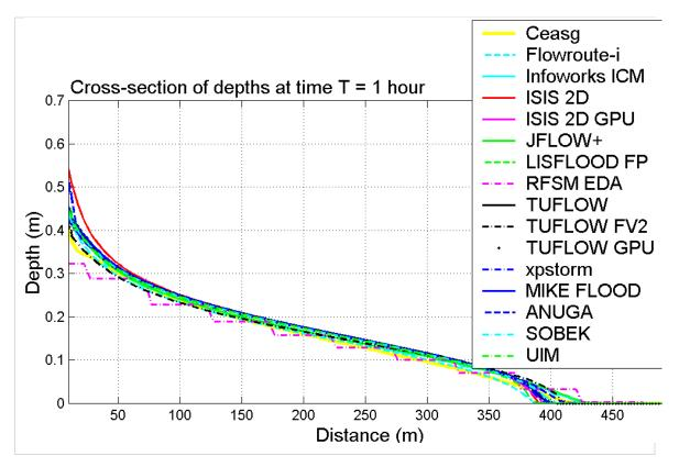
Figure 4.13 Cross-section of depths along the dashed line in Figure 4.12 at time t = 1h
