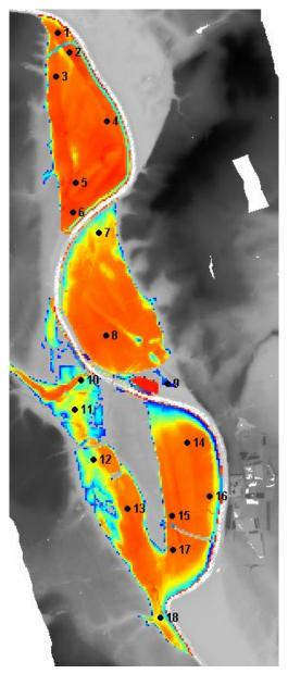
Figure 4.40 Peak depths predicted by ISIS Fast in Test 7
