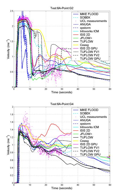
Figure 4.26 Velocities time series (results at a selection of points: G2 and G4)
