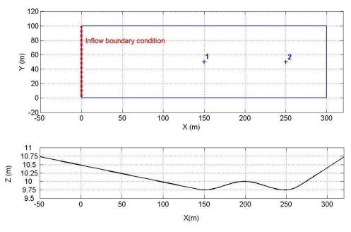
Figure A.5 Plan and profile of the DEM use in Test 3
