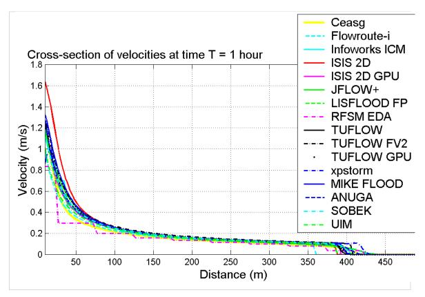
Figure 4.14 Cross-section of velocities along the same line as Figure 4.12 at time t = 1h
