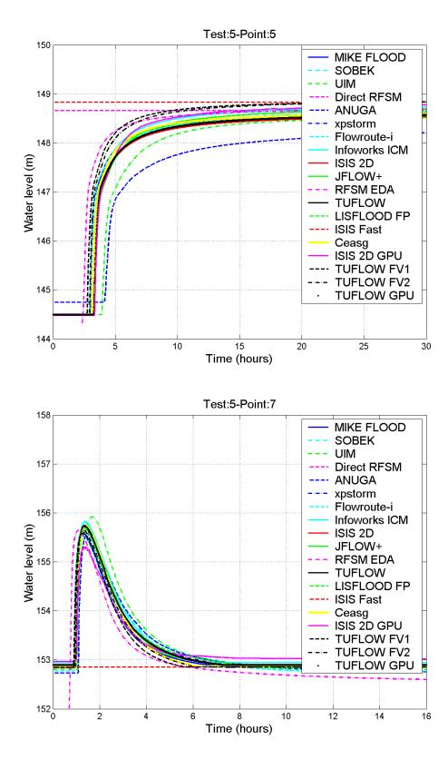
Figure 4.16 Water levels time series (results at a selection of points: 1, 3, 5 and 7)
