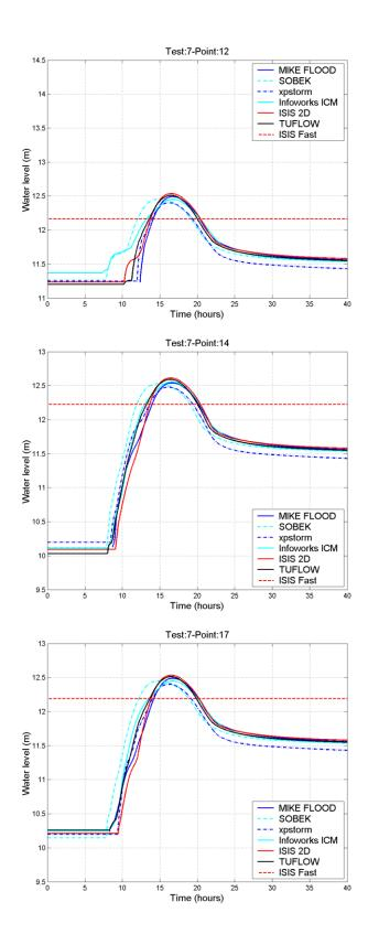
Figure 4.36 Water levels time series for floodplain 3
