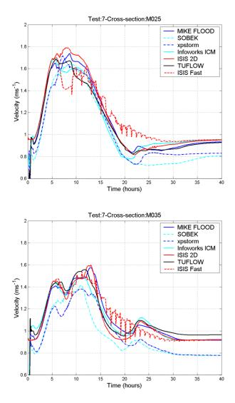
Figure 4.33 Velocities at river cross-sections M025, 35
