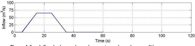
Figure A.6 Inflow hydrograph used as upstream boundary condition
