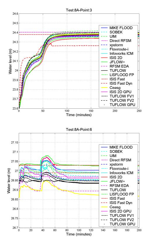
Figure 4.42 Water levels time series at points 1, 2, 3 and 6
