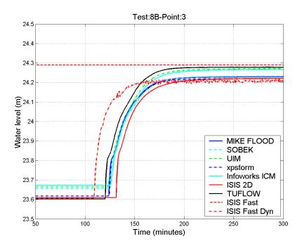
Figure 4.47 Water levels time series (results at 1, 2 and 3)
