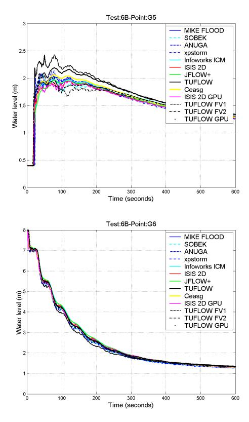
Figure 4.27 Water levels time series (results at a selection of points: G2, G4, G5 and G6)
