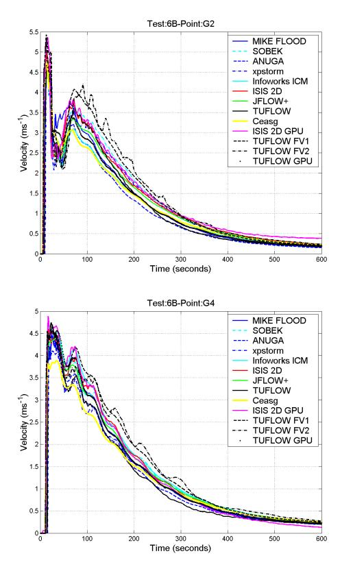
Figure 4.28 Velocities time series (results at a selection of points: G2 and G4)
