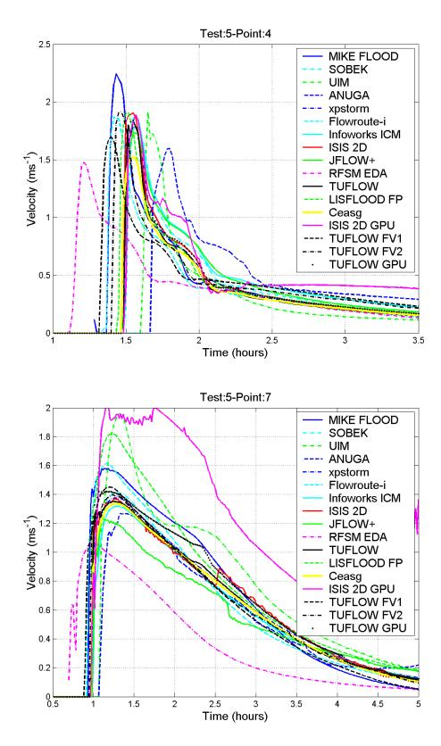
Figure 4.17 Velocities time series (results at a selection of points: 1, 3, 4 and 7)
