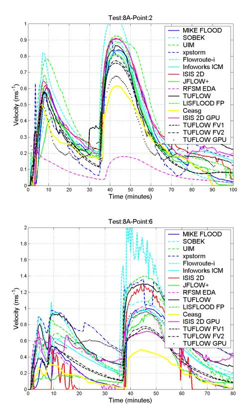
Figure 4.43 Velocities time series at points 2 and 6
