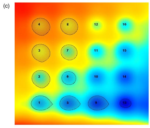
Figure 4.6 Final inundation extent as predicted by (b) ISIS Fast Dynamic, (c) RFSM Direct and (a) all except the latter two Notes: These figures were constructed by assuming a horizontal final water surface in each depression.
