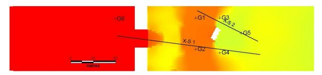
Figure 4.29 Plan view showing the hydraulic jump and the locations of the cross-sections (from a peak water level grid)
