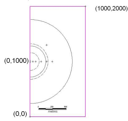
Figure A.7 Modelled domain, showing the location of the 20m inflow, six output points, and possible 10cm and 20cm contour lines at time 1h (dashed) and 3h (solid)
