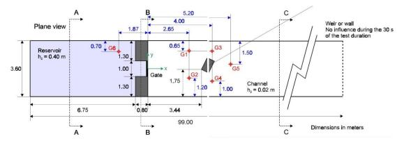
Figure 4.24 Set-up for Test 6A (adapted from Soares-Frazão and Zech 2002)
