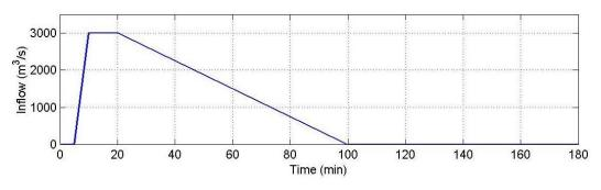
Figure A.10 Inflow hydrograph applied in Test 5
