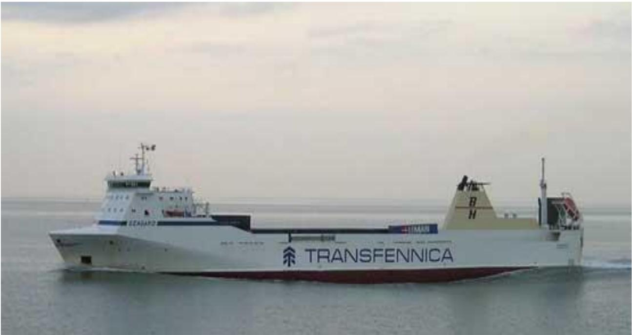
APP 5: FIGURE 2: Vessel experiencing significant 'squat' effect, as characterised by the water being 'drawn-down' in the area of its maximum vertical blockage point (advancing underwater cross-sectional area).
