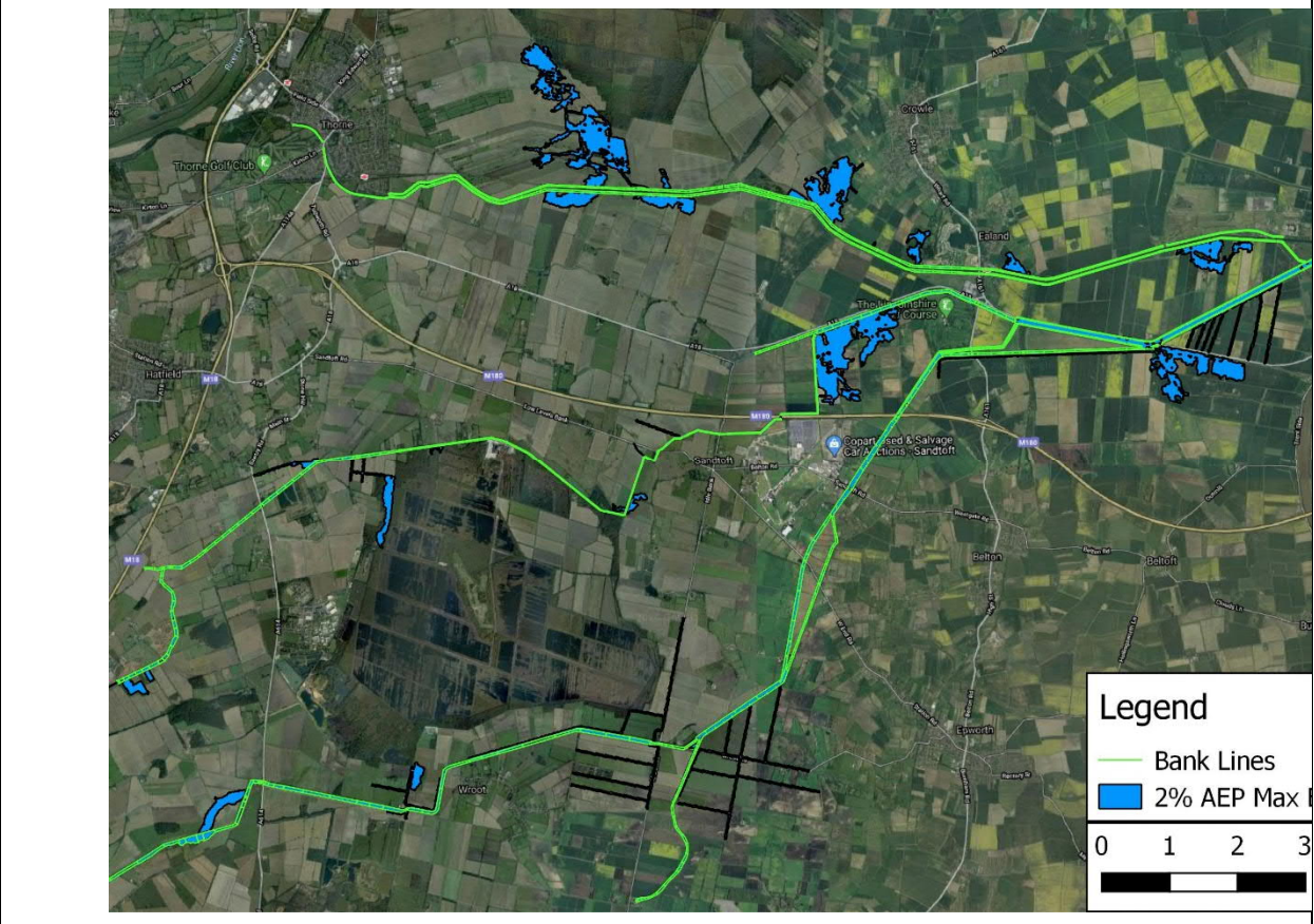
Figure 8: Lower Torne: 50% AEP flood extent and bank lines demonstrating areas where out of bank flooding occurs.
