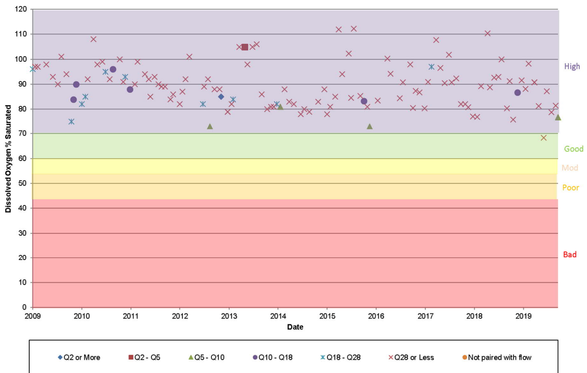
Figure 3.50 Dissolved oxygen (% saturation) in the River Maun at Whinney Hill (upstream site) (flow band on day of sampling from the Maun at Mansfield the Dykes) 2009 - 2019
