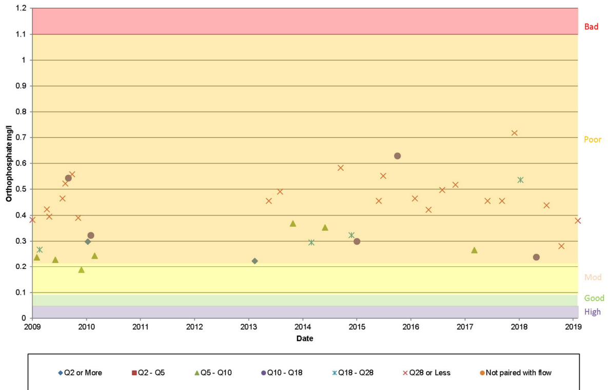
Figure 3.34 Orthophosphate concentrations in the Old Coates Dyke at Blyth (flow band on day of sampling from Old Coates Dyke at Blyth – 1.2km upstream) 2009 - 2019
