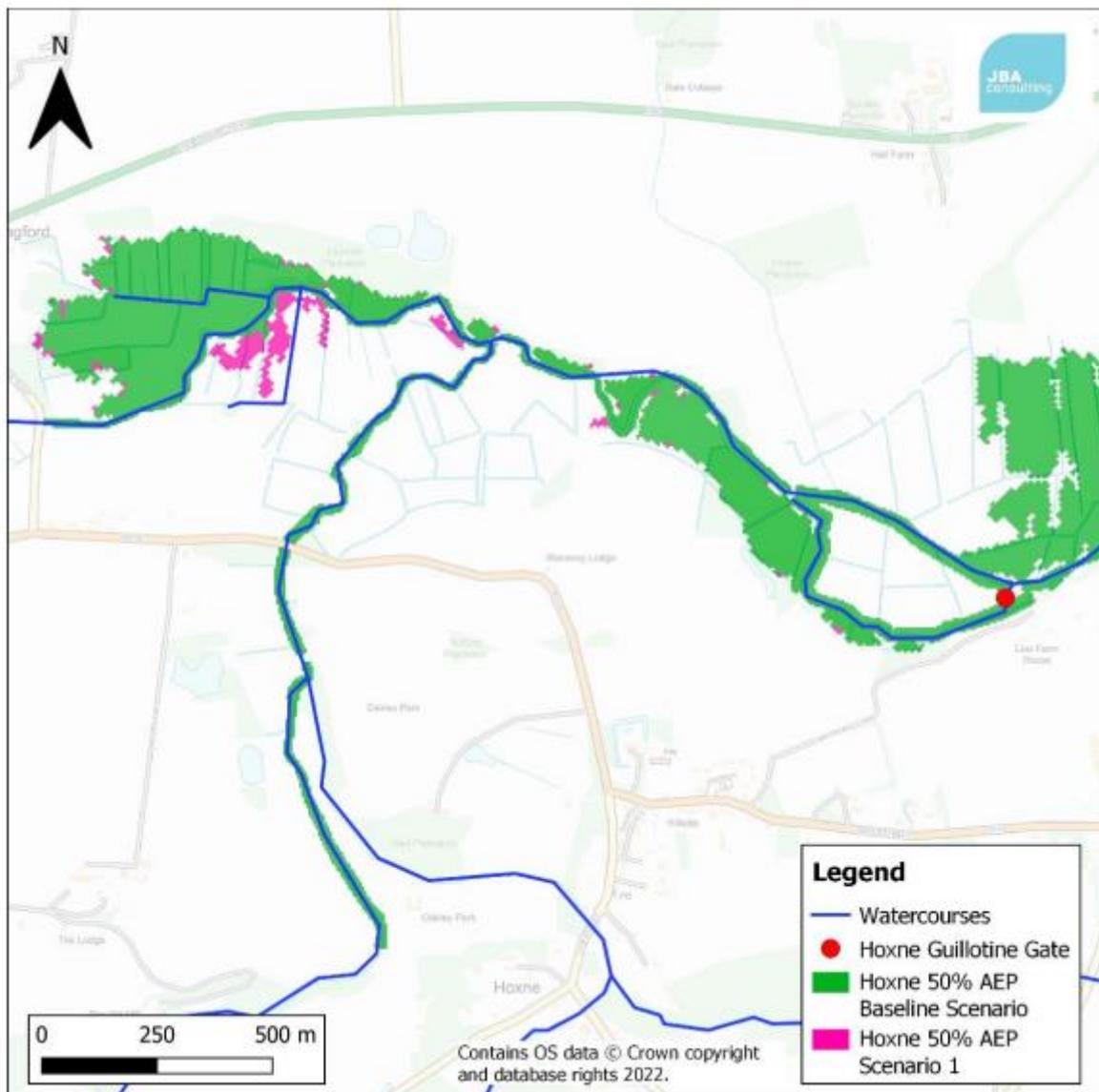
There is only a minor increase in flood extent in the 5% AEP event and during the 1% AEP event the increase is described as insignificant in the report. Increases in flood extent are located up to 2.6km upstream of the structure during the 50% AEP event, 1.67km upstream during the 5% AEP event and 1.18km during the 1% AEP event.
