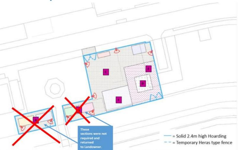
A = 4no 10x3m single stacked cabins, B = Staff & contractor parking area, C = Asphalt lorry parking & turning area, D = Hot box & asphalt skips, E = Asphalt & dumper access, F = Material Laydown Area.
