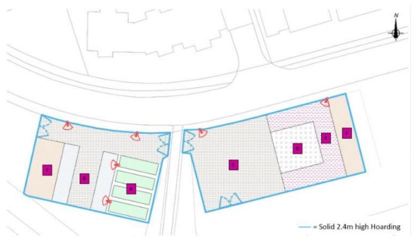
A = 4no 10x3m single stacked cabins, B = Staff & contractor parking area, C = Asphalt lorry parking & turning area, D = Hot box & asphalt skips, E = Asphalt & dumper access, F = Topsoil Storage bund.
