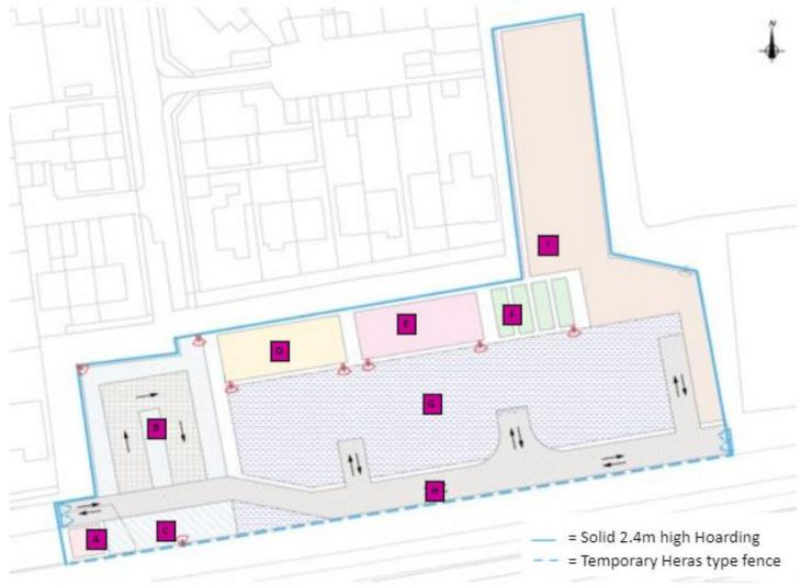
A = Gate House, B = Staff & Contractor Parking, C = <u>over flow</u> parking, D = 8 bay single storey modular office unit, E = 8 bay single storey modular welfare unit, F = Stores unit area (4no 10x3m units), G = Hardstanding area for material storage, precast working area, OSA/LSA storage area, H = 2 way access road, I = Topsoil storage bund.
