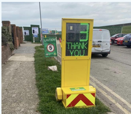
Speed activation unit
