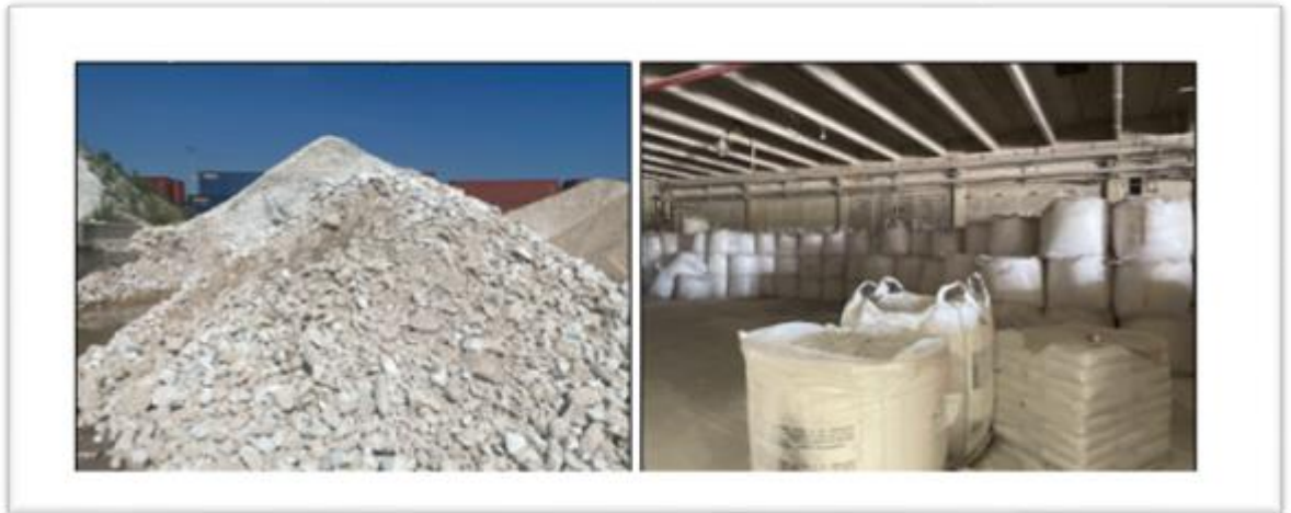
Figure 2.1 Brucite pile before milling down to D50 10 micron (left), final UM10 product in 1-tonne super sacks ready for shipment
