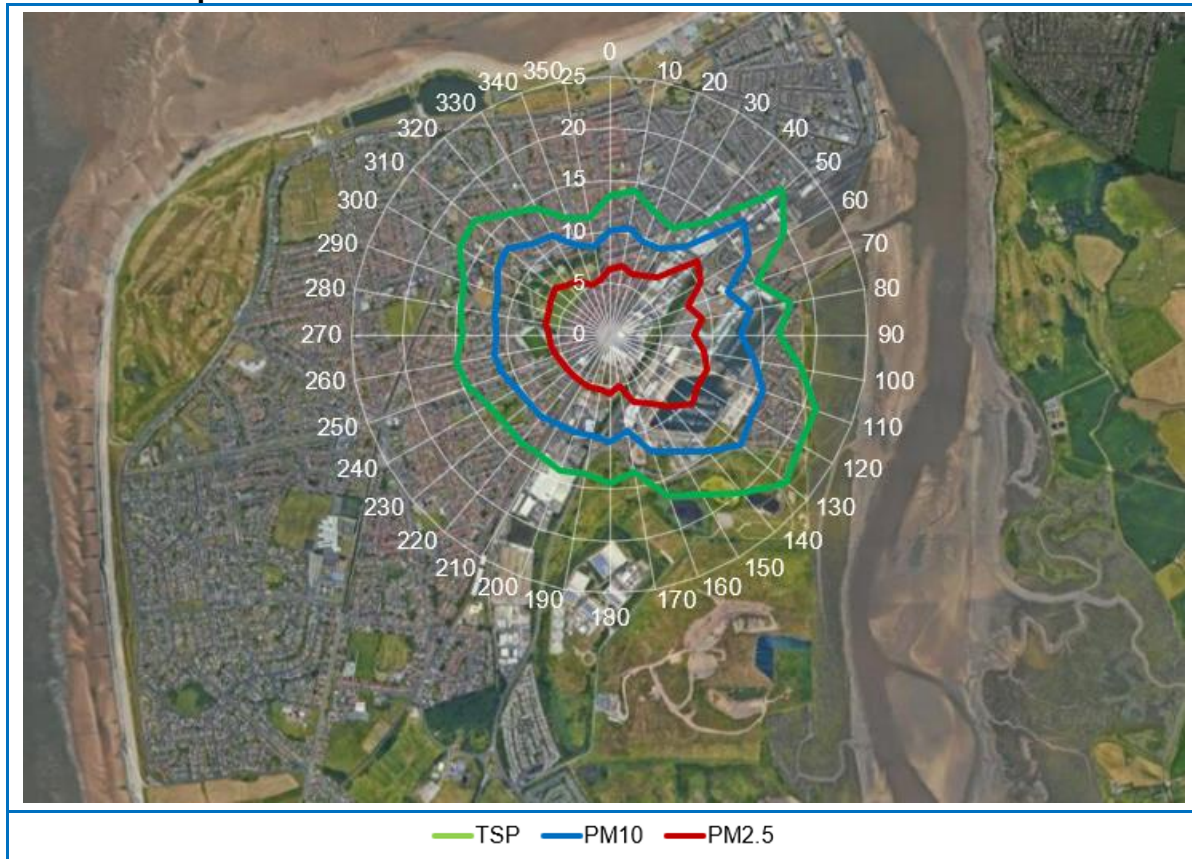
Figure 3.4.5: PM Concentration Rose ( \mu\text{g}/\text{m}^3 Mean Concentration) for each 10° Sector Overlain a Map of the Area.
